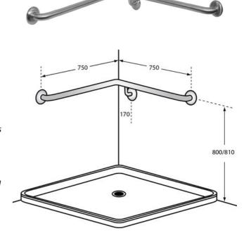
This product is AS1428.1 compliant (accessible compliant) when installed in accordance with the guidelines.
